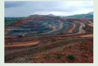
It is the first opencast uranium mine of the country and was commissioned in January 2009 with a capacity to produce 3500 tpd ore. Situated adjacent to Turamdih Mill, the deposit contains a moderately large reserve with very low uranium content. It is a conventional opencast mine using excavator-dumper combination. It has ore benches of 6m height, over burden/waste benches of 6m/12m height. The pit will attain the ultimate depth of 160m with ore to overburden ratio of 1:2.7.
